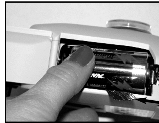
FIGURE E Installing the battery
