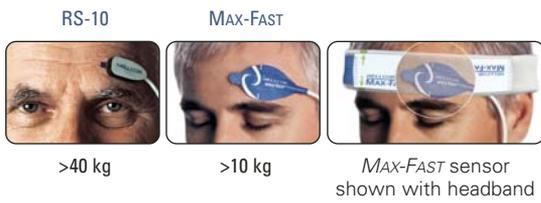
With unique calibration coefficients embedded in its digital memory chip, the *MAX-FAST* sensor is the forehead sensor of choice. It is more accurate than the earlier-generation RS-10 Forehead Sensor. Its SpO<sub>2</sub> accuracy level of  $\pm 2\%$  is comparable to most adhesive digit sensors. In addition, the *MAX-FAST* sensor has improved bandaging material and adhesive attachment compared with the RS-10.
